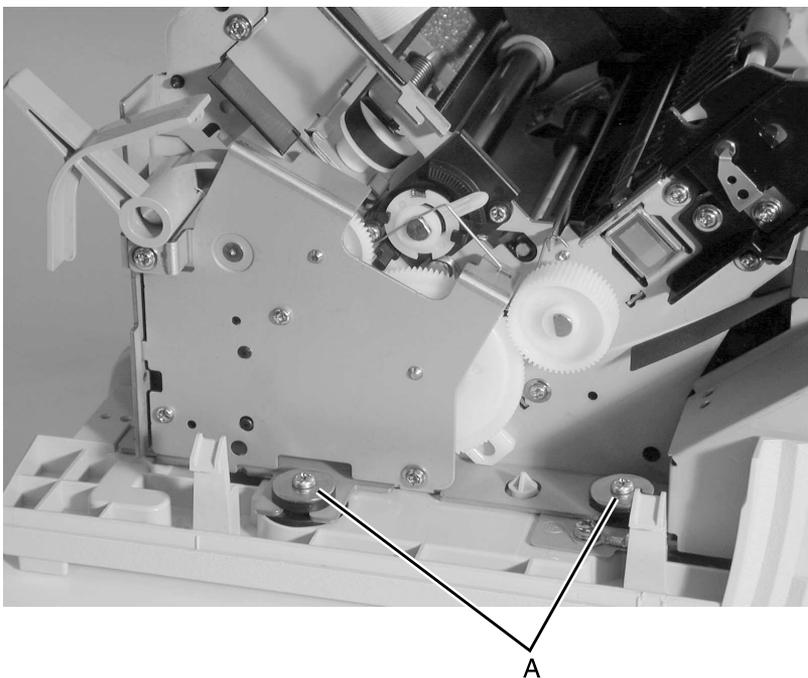
6. Remove the print unit from the bottom cover, by pulling up forcefully on both sides of the print unit.
