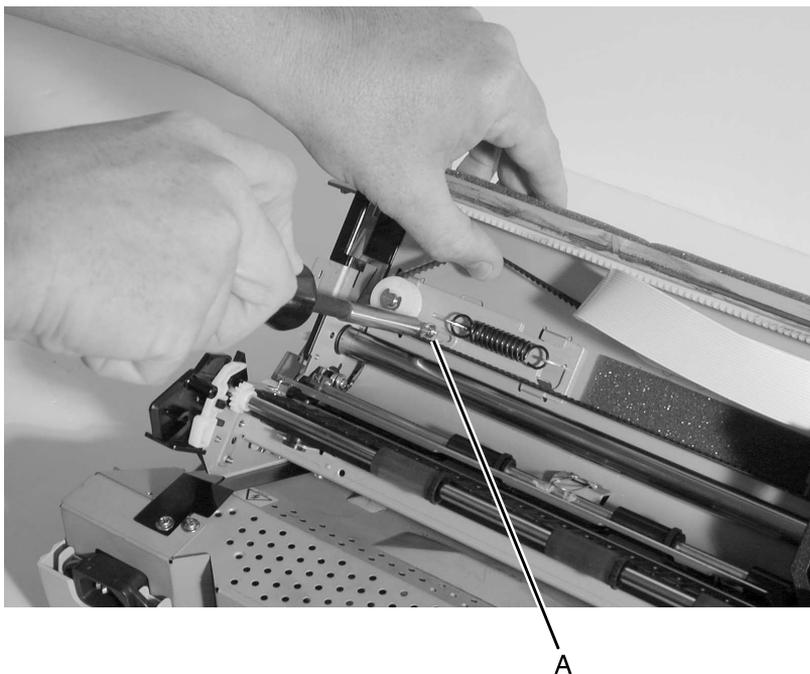
3. Slip the belt off the carrier motor pulley.
