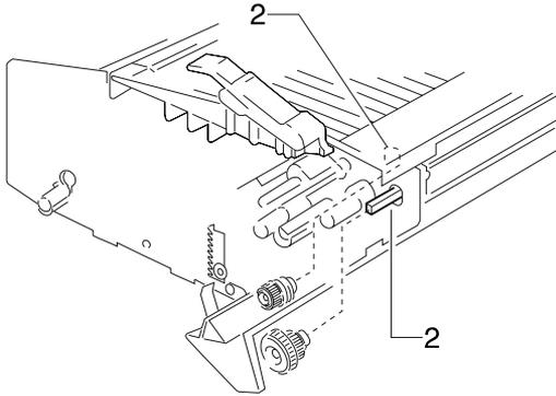
Gear mounting studs on the right ASF side frame [2].
