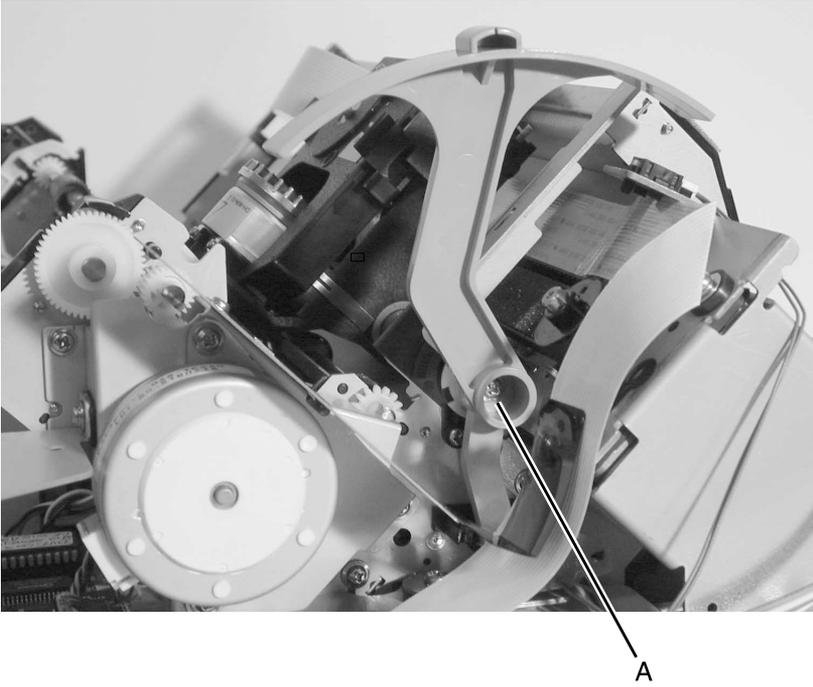
5. Remove the screw [A] securing the carrier motor bracket to the bottom cover.
