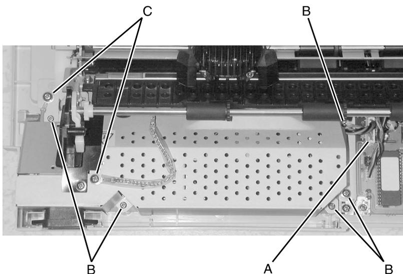
4. Disconnect the power supply cable [A].
