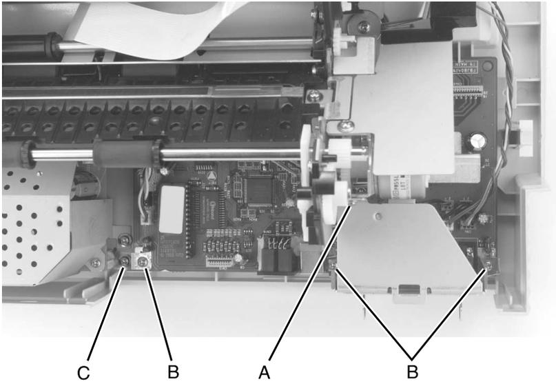
4. Remove the three screws [B] securing the logic board to the bottom cover. Take care not to lose the ground clips which must be replaced between the ground plate and the board.
