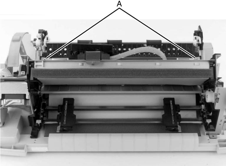
10. Remove the carrier motor bracket. Go to **“Carrier, Motor Assembly Removal”** on page 4-21.
