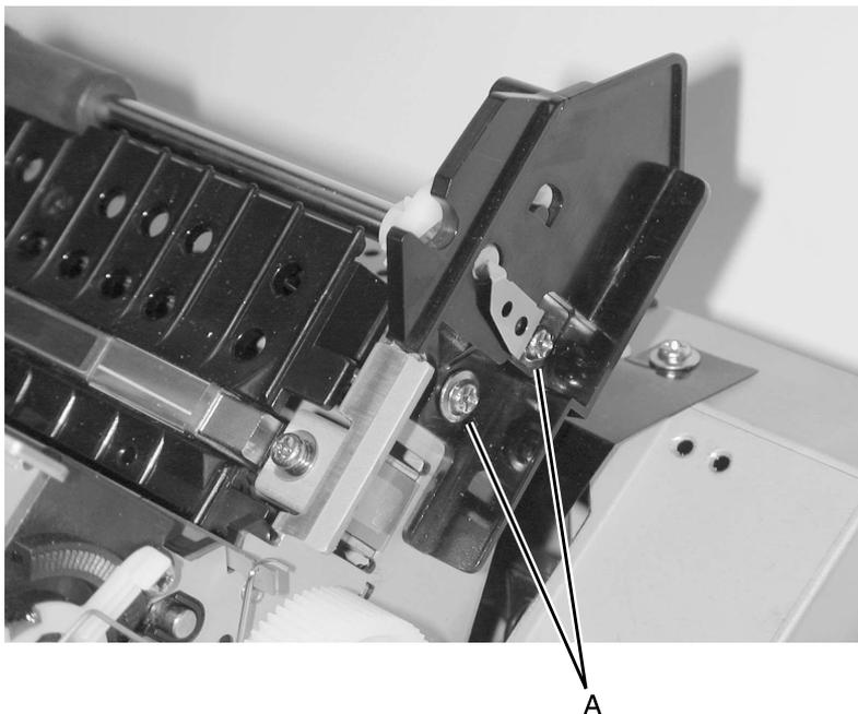
5. Pull the upper feed roller from the left bracket and out of the printer.
