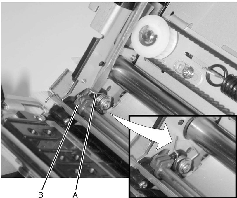
8. Slide the carrier to the right side of the printer.
