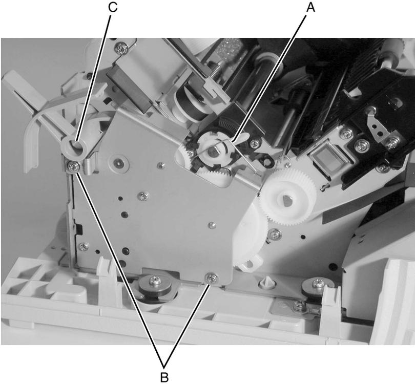
3. Remove the two screws and washers [B] from the sub frame.
