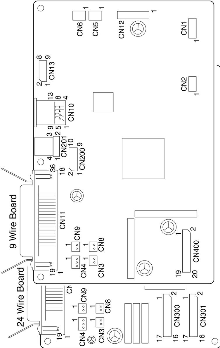
**Logic Board - Dual Tractor Cable (9w & 24w)**
