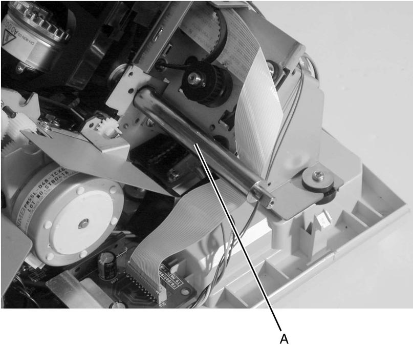
10. Remove the carrier from the printer.
