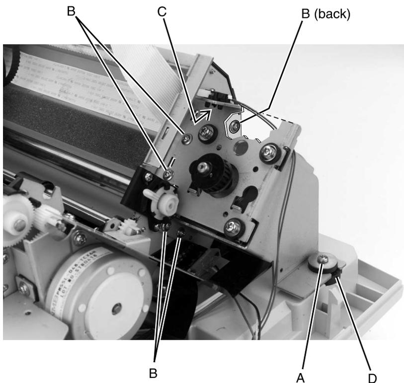
6. Disconnect the printhead cable from the logic board and move it back and out of the way, as shown.
