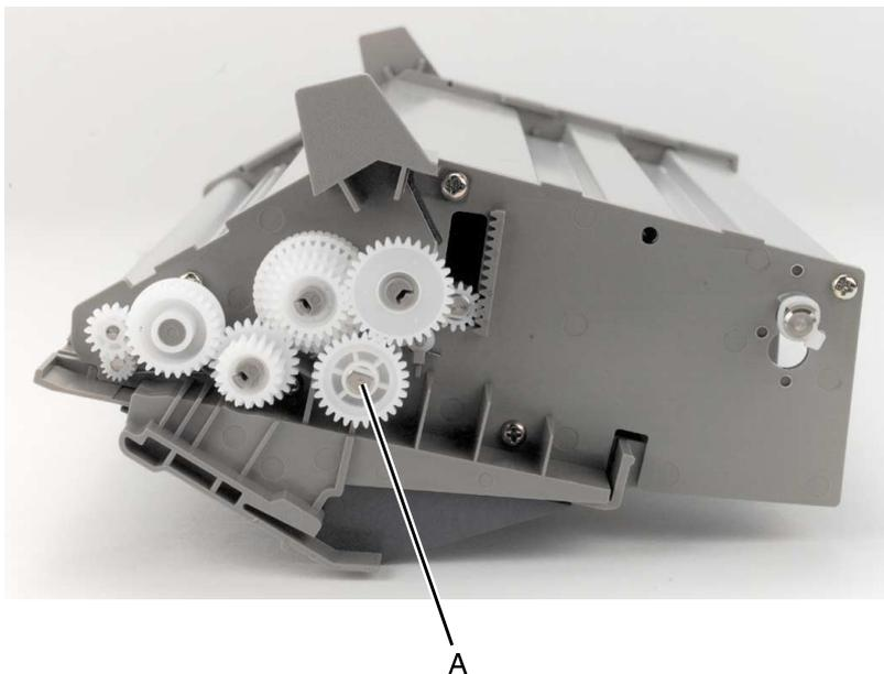
3. Release the idler gear latch and remove the idler gear.
