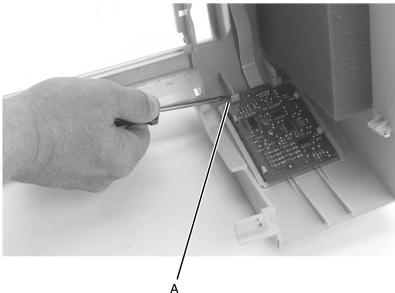
4. While holding the latches down, push the operator panel out of the top cover, toward the bottom of the cover.
