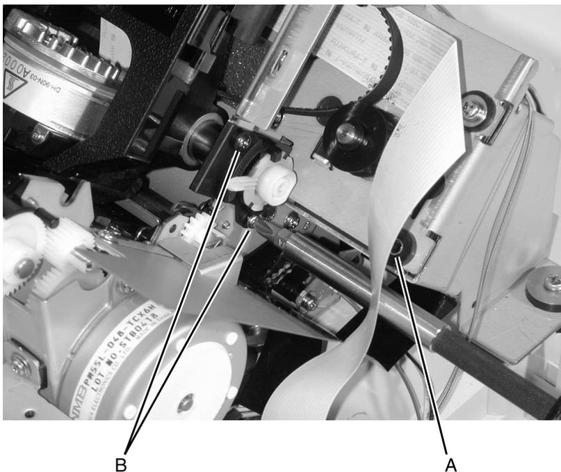
8. Remove the E-clip from the right side of the carrier shaft.
