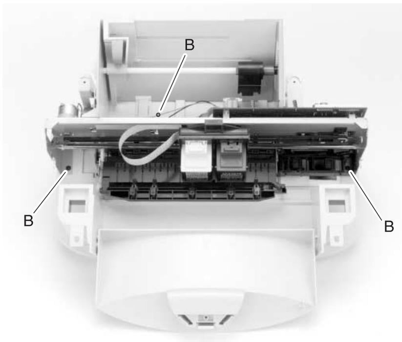
8. Slide the print engine forward and remove.
