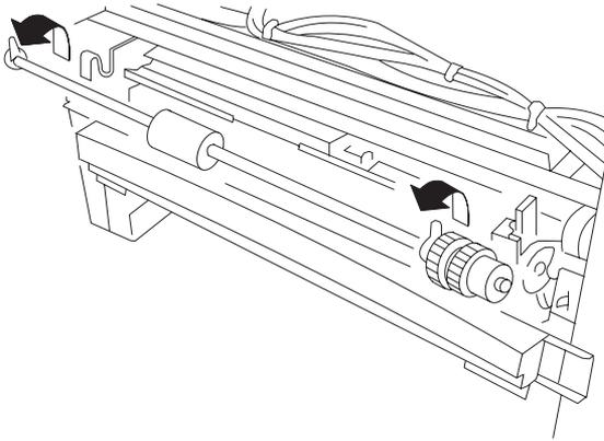
4. Remove the E-ring and MPF clutch.
