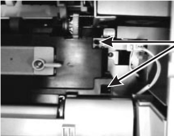
6. Lift the fuser out of the printer.
