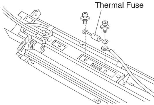
4. Remove the temperature fuse, (silver screw with washer).
