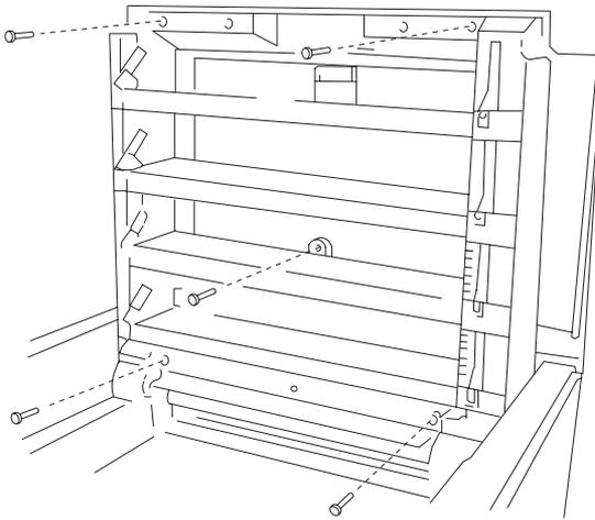
4. Remove the second paper cassette connector cover on the bottom of the rear cover.
