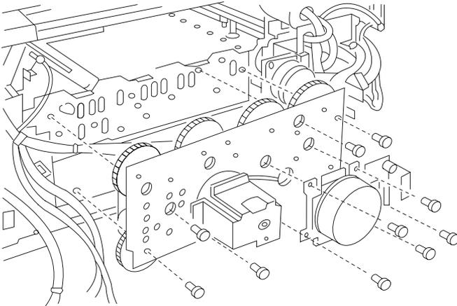
**Installation Note:** When you connect the terminals be sure to connect them to the correct position. After the terminals are connected, firmly insert the insulating cover.
