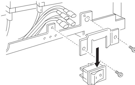
Installation Note: When you connect the terminals be sure to connect them to the correct position. Also, after the terminals are connected, firmly insert the insulating cover.
