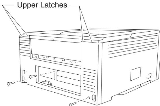
8. Lift the cover over the top latches and lift back.
