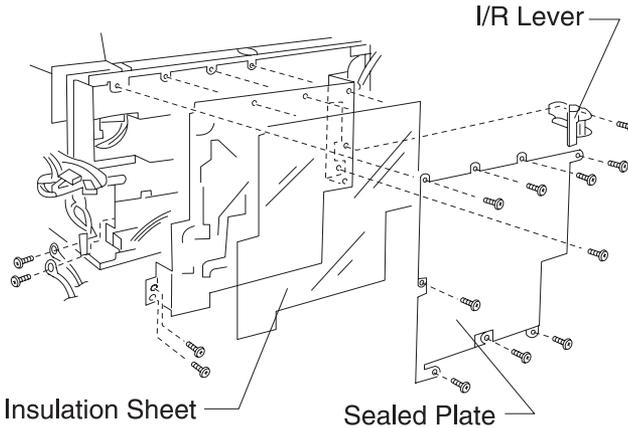
**Note:** Be sure the I/R lever works correctly after you reassemble.
