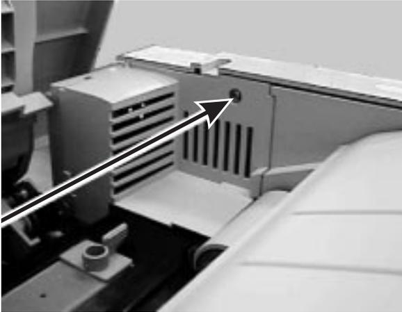
2. Remove left-rear sub-cover mounting screw and remove the cover.
