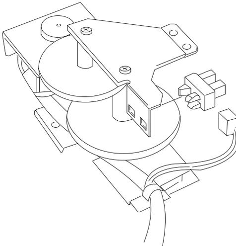
5. Disconnect the BUD motor connector and remove the 2 mounting screws. Remove the motor.
