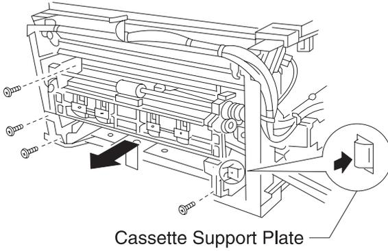
11. Remove the turn guide, (4 screws).
