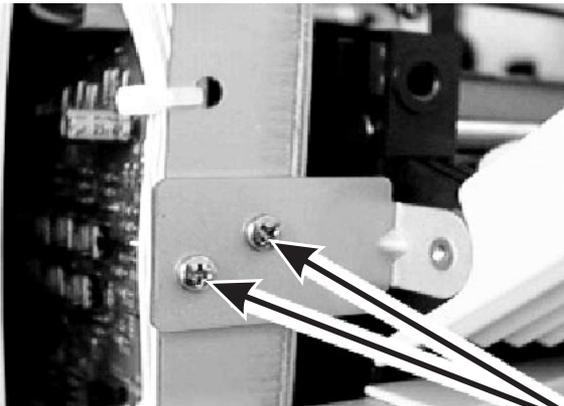
4. Remove the bearing stoppers from each side of the MPF(U). Release and turn the bearing position clips 90 degrees toward the front.
