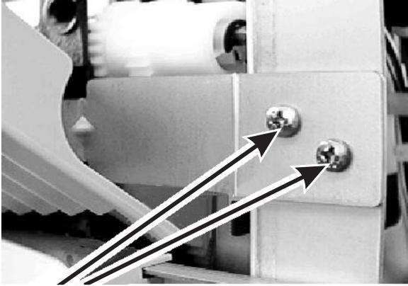
3. Remove the left MPF plate, (2 screws).
