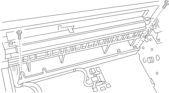
5. Remove the front sub-cover, (2 screws).
