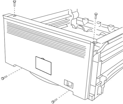
2. Remove the 2 screws that mount the left side sub-cover.
