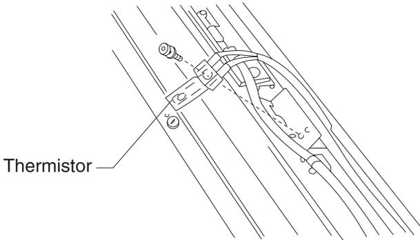
7. Remove the thermistor, (1 silver screw with washer).
