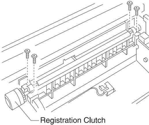
When you reassemble, put conductive grease on the contact portion between the shaft of the registration roll unit and registration roller ground plate.
