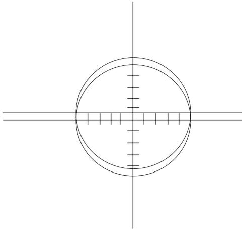
When the Y value is correctly adjusted the magenta radar image should look like the following example. The Theta adjustment is done in the same manner as the Y except theta values are taken from the right side of the test pages.
