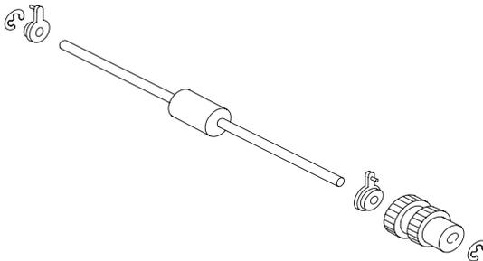
Assembly Note: Put conductive grease on the contact portion between the shaft of the resist roll and the resist roller ground plate.
