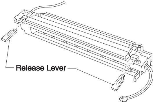
2. Remove the 2 release levers and stopper screws.
