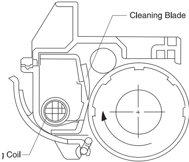
A rotating coil in the waste toner conveyance assembly conveys the scraped-off toner to the waste toner bag.
