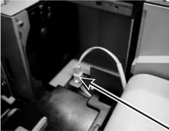
4. Remove the harness connector from the power supply board.
