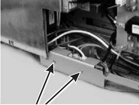
4. Remove the HDRV board from the HK bracket, (2 screws).
