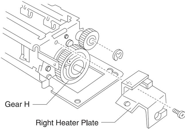
5. Remove the fuser roller.
