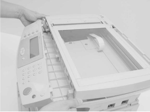
9. Lift the scanner cover, and thread cable through chimney to remove.
