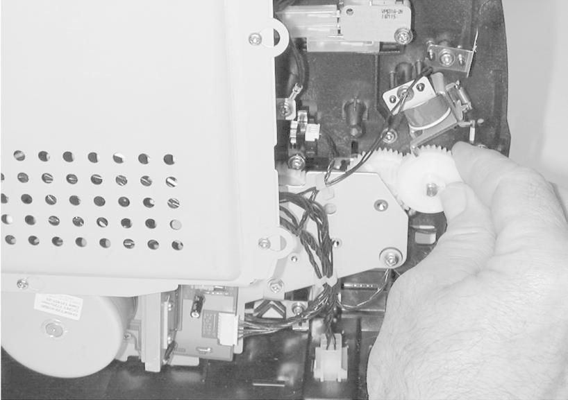
4. Remove the gear train assembly. See **“Main drive assembly removal”** on **page 4-44** for more information.
