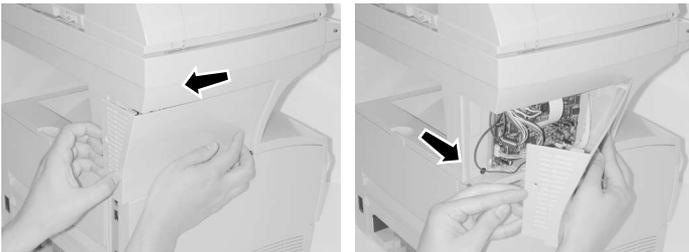
5. Remove two screws in the scanner base [A].
