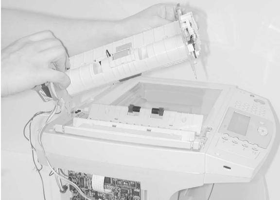
**Note:** Perform the scanner calibration and scanner registration procedures after replacing this part.
