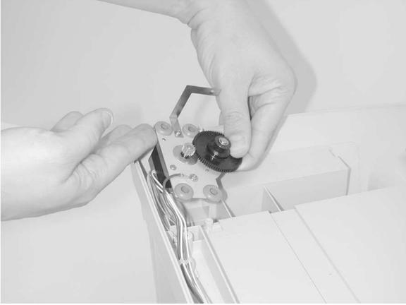
**Note:** This plate needs to be attached to the new flatbed motor.
