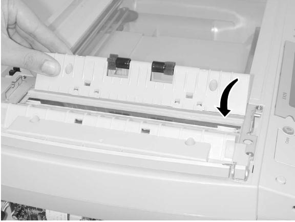
**Note:** Reinstall: ensure extended edge of the R2 idler [A] is slipped under the scanner glass.
