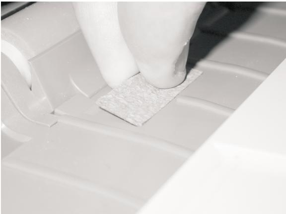
**Note:** To avoid jams, in the ADF, ensure the leading edge of the pick pad is pressed firmly into the guide.
