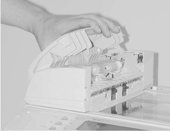
4. Push with a screwdriver to release two tabs [A].
