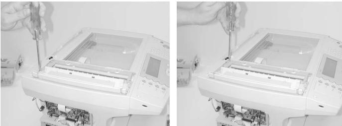
8. Pull idler and bracket away from scanner and remove.
